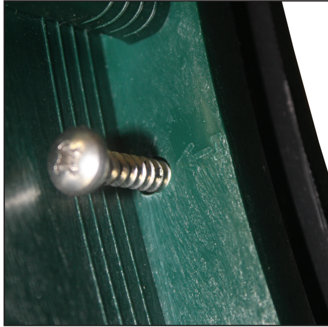
4. Tighten (10) ten #14 x 1.5" stainless steel Phillips head screws in a star pattern onto the RTR.
